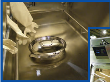
Manway Transfer Ports and Material Trolley Rail
