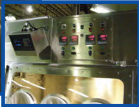
Programmable Logic Controls & Alarm System
