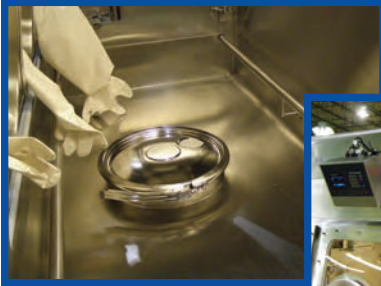
Manway Transfer Ports and Material Trolley Rail
